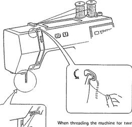
When threading the machine for twin needle seving follow this chart making sure you separate the threads, placing one in each thread guide on the needle bar.
